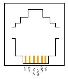
Serial Cable Permanent Connections
